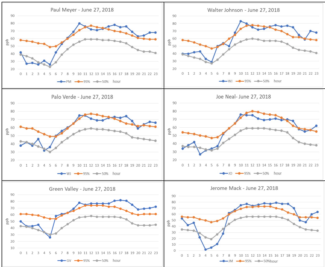
Figure 4-11. 5-Year Hourly Seasonal 95 th & 50 th Percentiles for O 3 and Observed O 3 on June 27.
